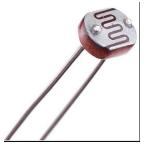
Although a semiconductor material is used for these photoresistors, they are purely passive devices because they do not possess a PN junction, and this separates them from other photodetectors like photodiodes and phototransistors.
